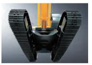
Improved box-like structure has lower barycenter and goodstability. The enhanced four wheels and crawler is suitable for harsh environments.
