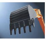
The bucket is made of wear-resistant material, which has a strong structural strength. Its big capacity improves the operation efficiency.
