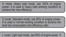
is used for light work, like clean up the ground.
